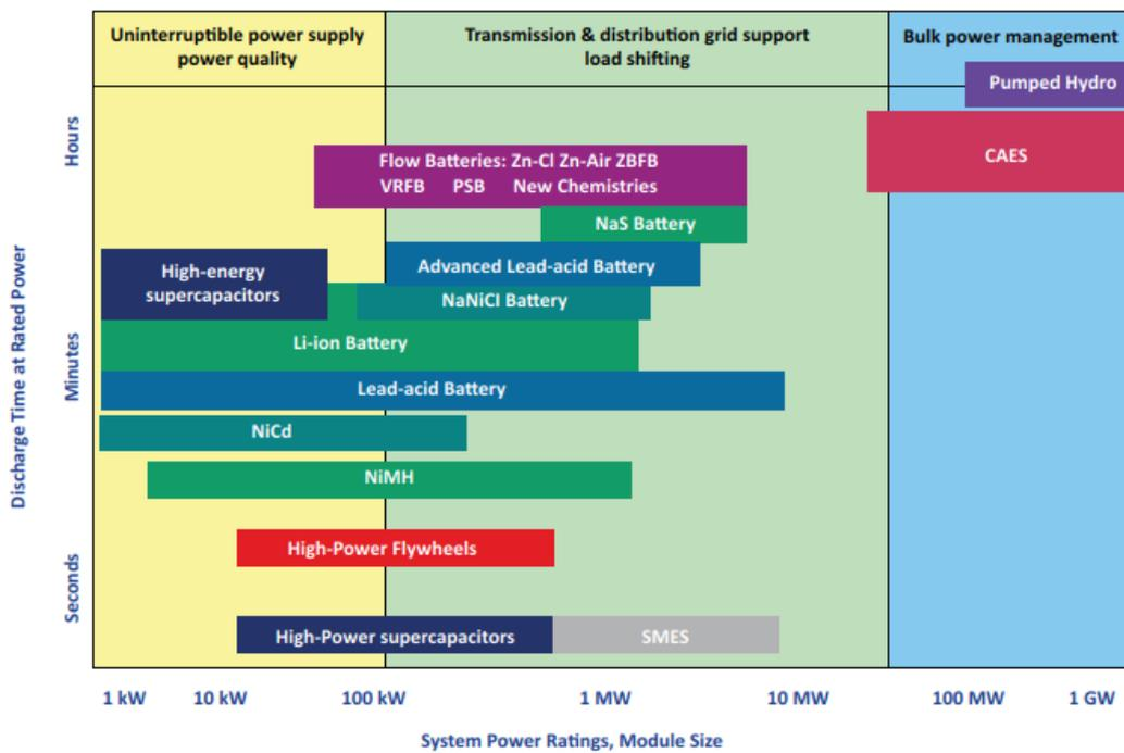
As it can be seen from the Ragone plot, chemical energy storage (batteries) covers a wide range of areas under the plot which signifies that battery storage is suitable for most of the applications.
